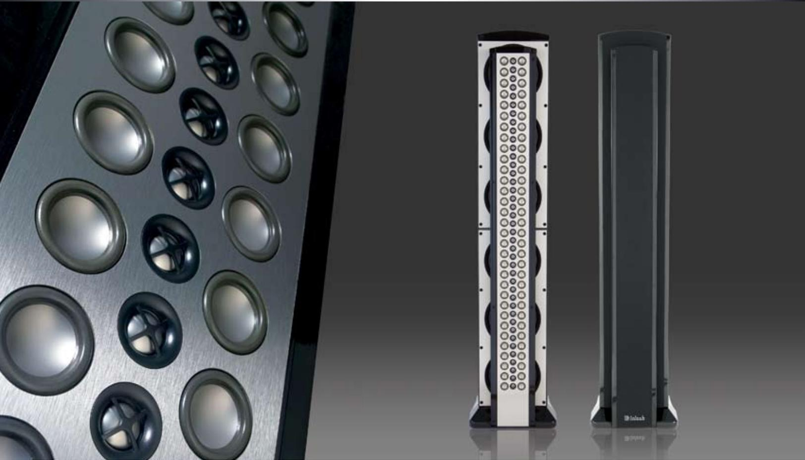
The XRT2K system is the speaker that speaker engineers have always dreamed of designing and building. McIntosh engineers made the dream come true with a three-way dual column design meticulously housing forty tweeters, sixty-four midrange and six woofers. All elements are chosen for use with high power amplifiers up to 2,000 watts.
