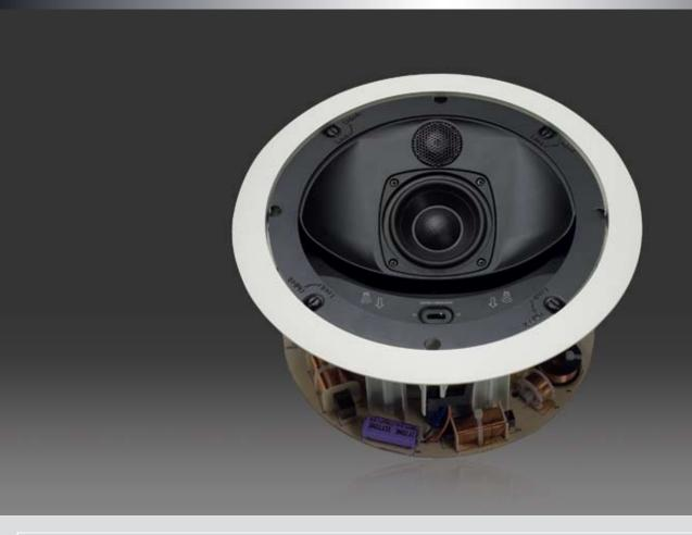
The CS100 is a 3-Way speaker designed for in-ceiling installation. One 8" Copolymer Cone Woofer, a 3-1/2" Neo Copolymer cone midrange and a 1" aluminum dome tweeter are neatly designed into the 12-7/16" diameter frame. The unique design of the CS100 allows for L/R applications, L/C/R and/or surround sound.
