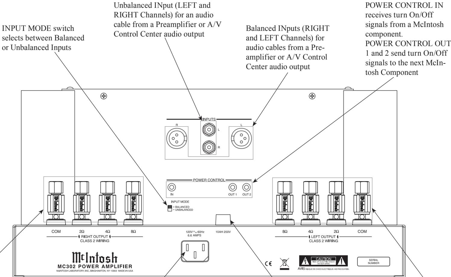
INPUT MODE switch selects between Balanced or Unbalanced Inputs
