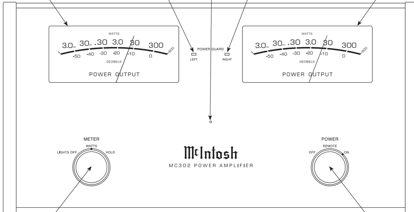
METER Switch selects the display modes of the Power Output Meter and Meter Illumination
