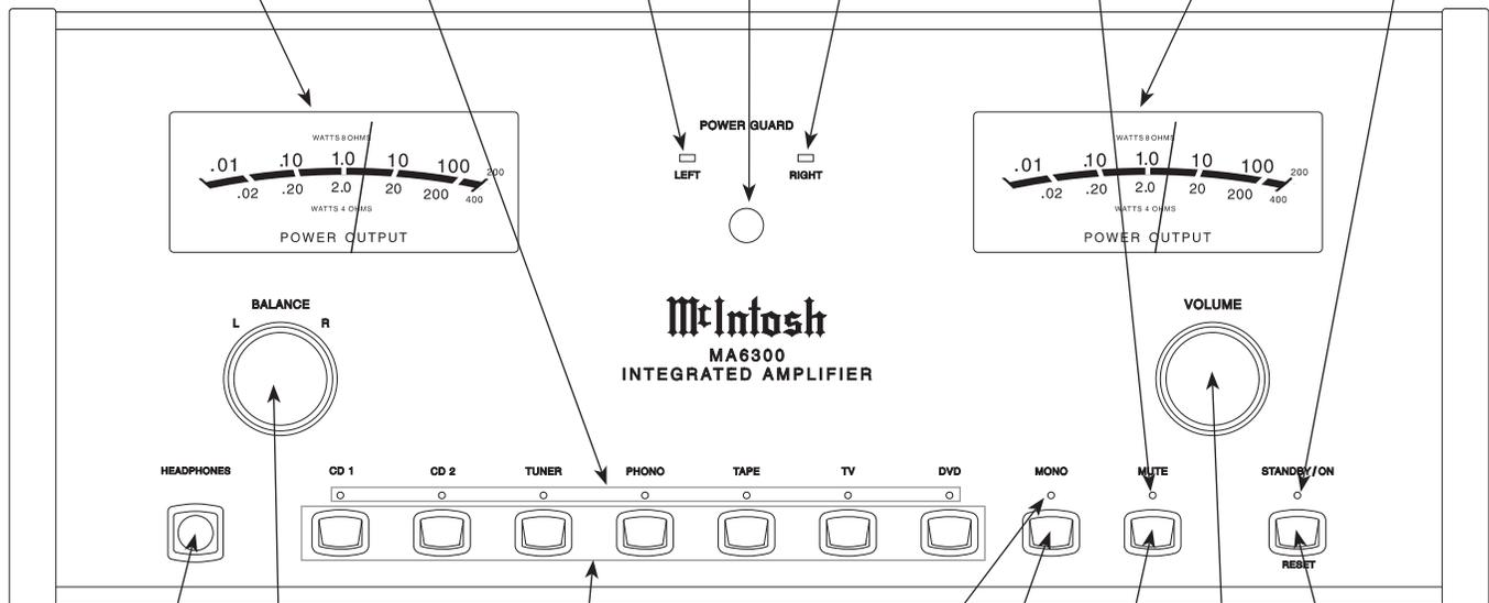
BALANCE Control allows adjustment of the relative volume balance between channels
