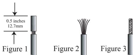
*Note: If desired, the twisted ends can be tinned with solder to keep the strands together, or attach spade lug and/or banana connector.*
