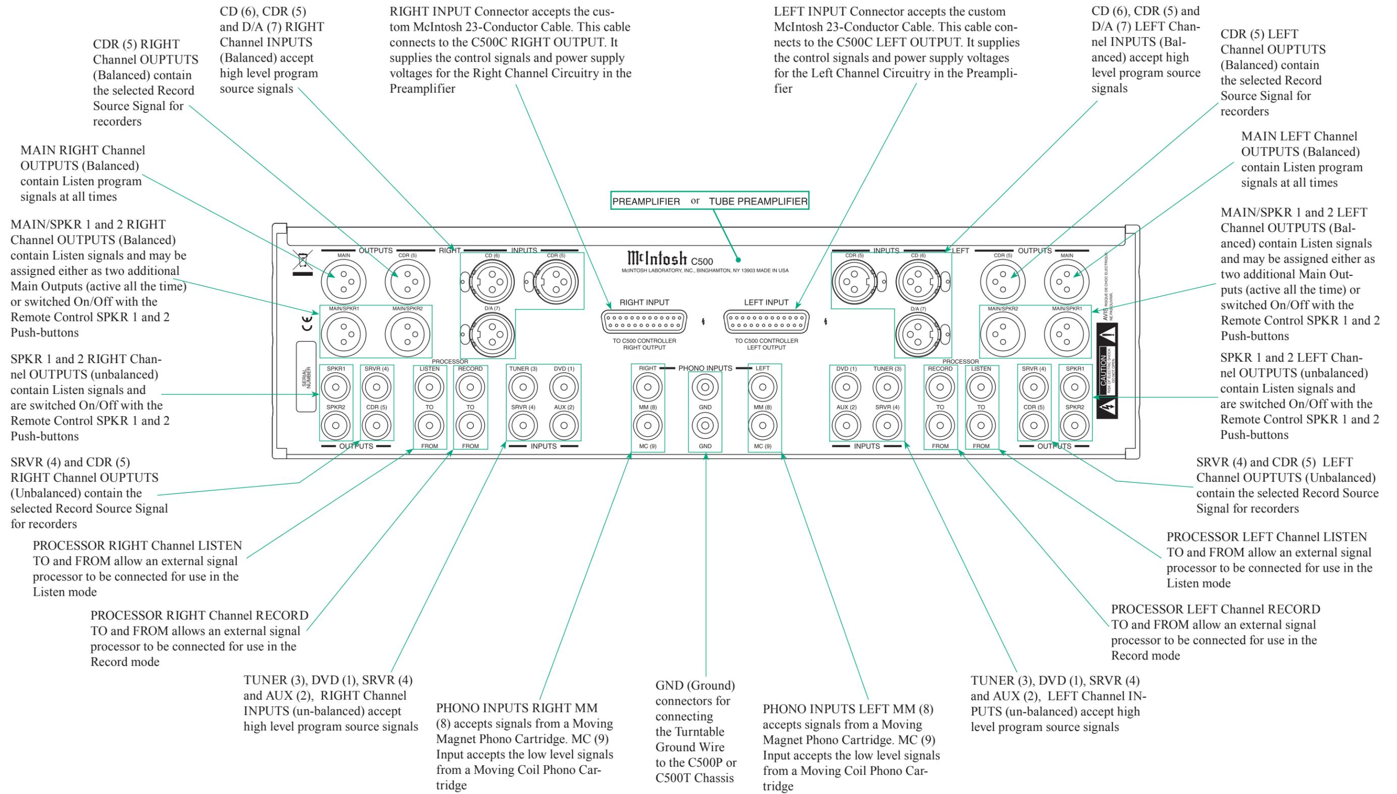
CD (6), CDR (5) and D/A (7) RIGHT Channel INPUTS (Balanced) accept high level program source signals
